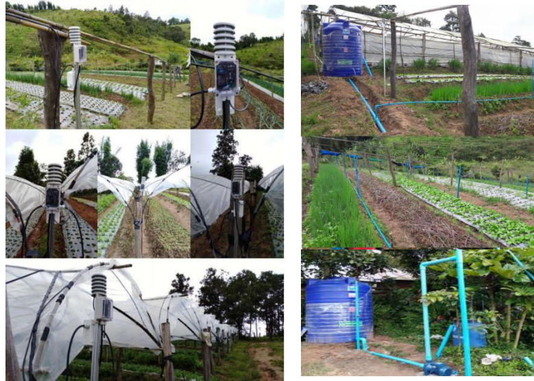
Figure 11: Setting up IoT sensors into the farm for irrigation, Chiang Mai, Thailand
